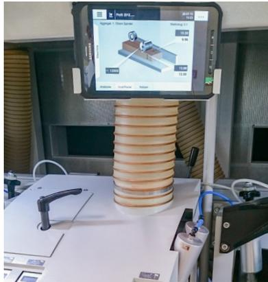
SmartTouch offers the display of setup information on a mobile tablet in addition to the main control unit. In this manner the operator has all relevant setup information in full view at the location where needed.
