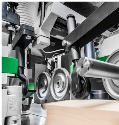
The top pressure roller opposite the left spindle only needs to be adjusted to the tool cutting circle once. When changing the width of the workpiece, the roller moves with the left spindle!
