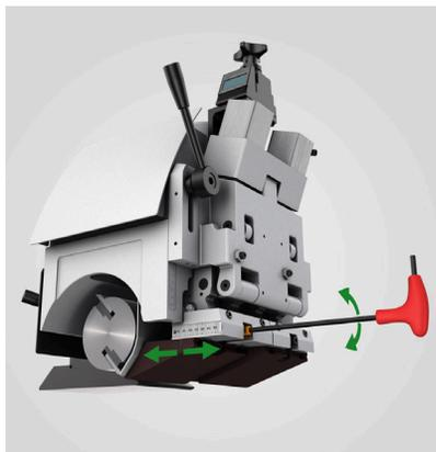
The chip breaker in front of the top spindle pivots away from the tool to avoid a collision. Due to the EasySet adjustment the chip breaker can be adjusted very simply to the tool cutting circle.
