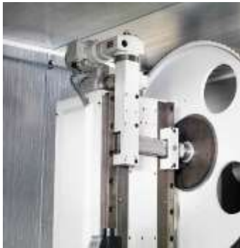
Picture 2: Tilt function of the upper saw wheel.
